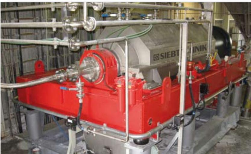
The DZ series can also be supplied in a vapor-tight and gastight design. For these applications, the product housings are manufactured in two pieces and sealed with chamber rings. The geometry of the rotating parts is designed for the specific separation requirement. The rotating assembly is carried by pedestal bearings located outside the product housing. Machines with bowl diameters greater than 1000 mm are standard design in the DZ series.
